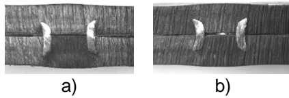
Figure 4 Cross-section of two different double-sided self-pierce riveted joints obtained ( h_0 = 8 mm and \alpha = 45^\circ ) with a) sharp chamfered ends r_f \cong 0 mm; b) blunt chamfered ends r_f \cong 0.2 mm.
